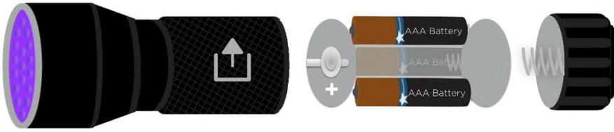
Insert the battery compartment into the flashlight with the '+' side facing towards the front of the flashlight
