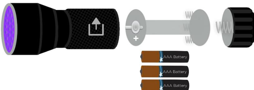
Install the 3 AAA Batteries into the battery holder by placing the negative side of the battery on the spring and pushing the positive side of the battery into the compartment with the '+' on it. Repeat for all 3 batteries.
